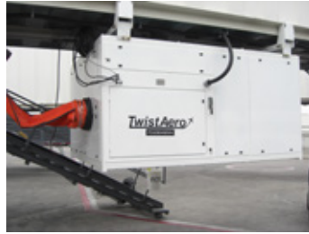
Air Handler Units (AHU)
